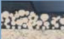
Maintenance-free, long-life sliding contact surfaces Sinter bronze composite
